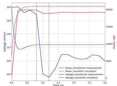
Results at the RE-Lab: Power and voltage at the transformer in the co-simulation (solid) and in the monolithic simulation (dotted).
