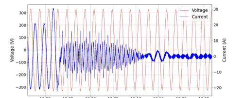
PV inverter measured EMT voltage and current during transient event
