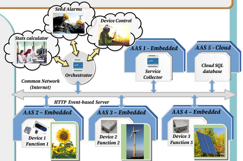
Figure 1: Basic AAS-based Orchestrator, Service collector and connected device
