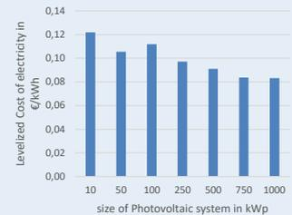
Fig. 3: Levelized cost of electricity
