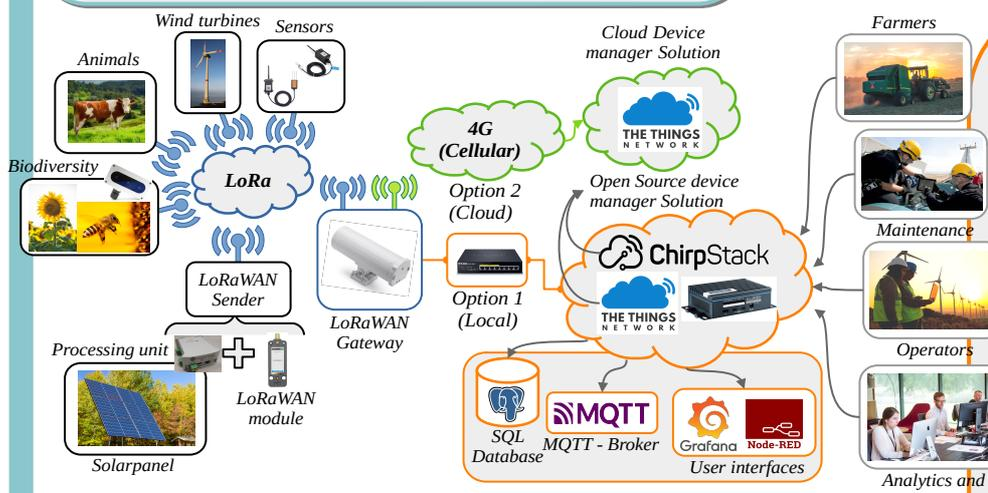
Figure 1: Deployed infrastructure for data collection according to the Technical Requirements of the Table 1
